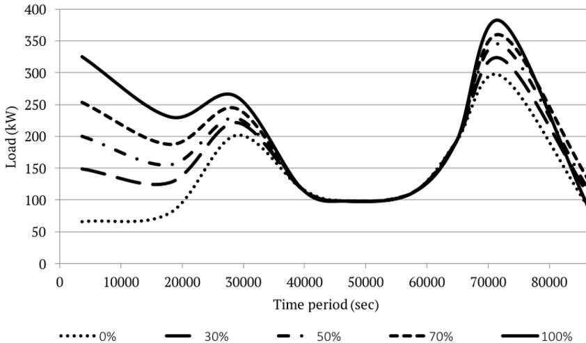
Figure 4.8: Load increase with different levels of EV penetration
