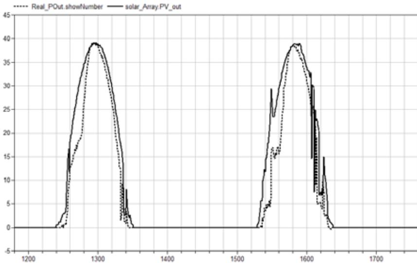
Figure 4.11: Simulated (Solid) vs Real (dotted) power (in kW) output from the PV array
