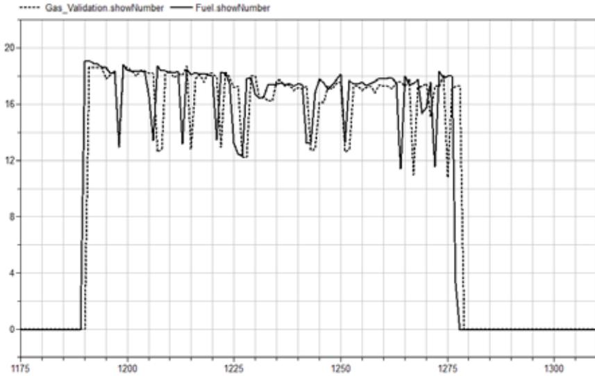
Figure 4.10: Simulated (solid) vs real (dotted) results for a daily profile for the C65 ICHP
