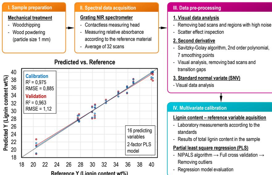
Figure 2. Spectroscopy work flow, Predicted vs. Reference plot for resulting PLS model
