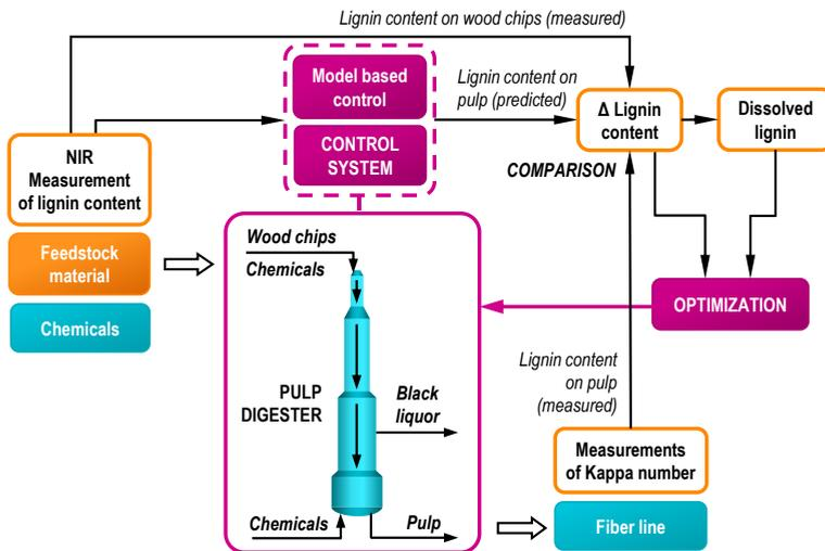
Figure 1. Scheme of pulping process with suggested integration of online NIR measurements
