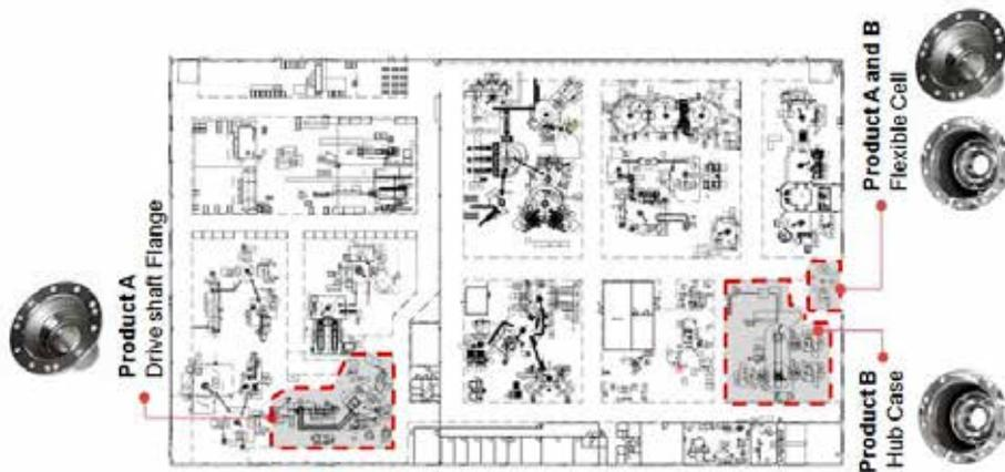
*Figure 10 – Two dedicated production cells and a flexible one to achieve volume flexibility at case company A*
