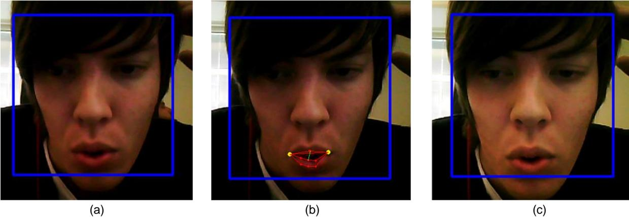
**Fig. 23.** The image shows that the system sometimes may have problem extracting the facial features. (b) show when the features are extracted correctly. But in (a) and (c) the feature extraction fails because the mouth could not be detected. If this would happen to many times in the images for the breath detection sequence it would result in a false negative result, meaning that a real breath was believed to be a false one.
