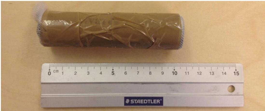
**Fig. 18.** The image shows a carbon filter that could be used to potentially be able to fool the breath test of an alcolock device.
