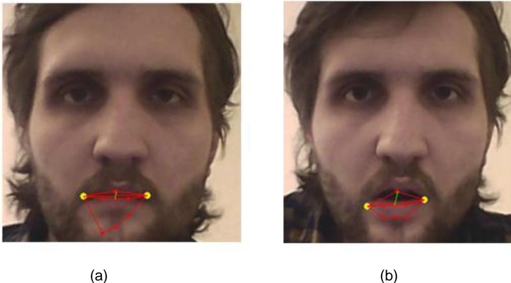
**Fig. 25.** This image shows the effects of facial hair on the tracking. In (a) the facial hair below the mouth causes the contour extraction for the lower lip tracking to make a faulty decision, the color difference of the lower lip and the facial hair may be too similar. In (b) the edge detecting of the corner detection mistakenly tracks the facial hair in the corner area.
