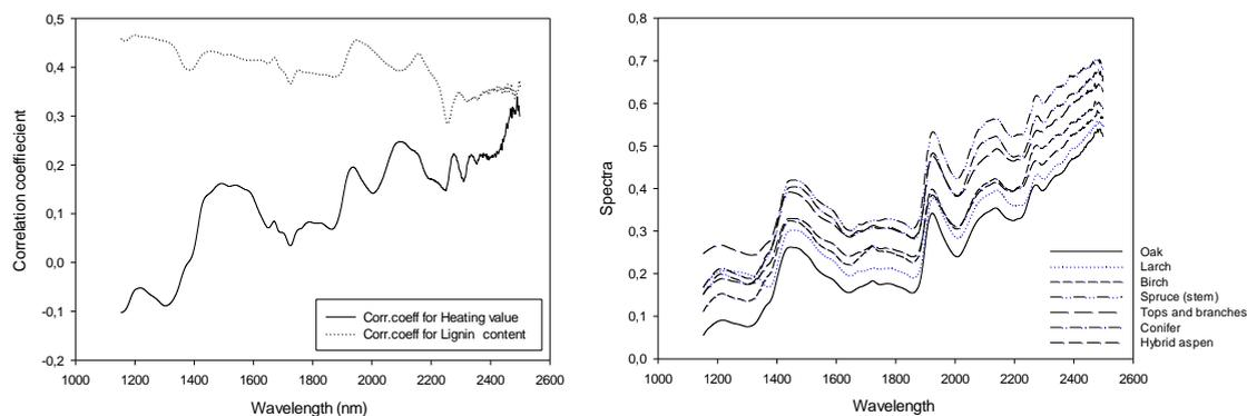
Fig. 1. (a) Correlation coefficients for NIR spectra vs heating value and lignin; (b) Comparison of NIR spectra for a selection of the wood samples analysed in the study
