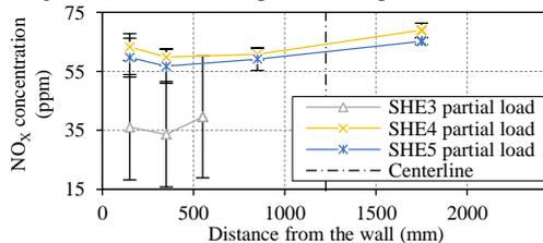
Fig. 9. NO<sub>x</sub> concentration profile – air preheaters
