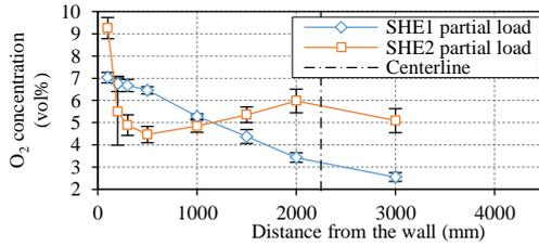
Fig. 3. O<sub>2</sub> concentration profile – side walls of the furnace
