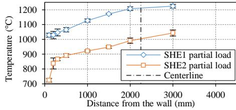
Fig. 2. Temperature profile – side walls of the furnace
