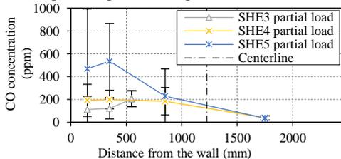
Fig. 8. CO concentration profile – air preheaters
