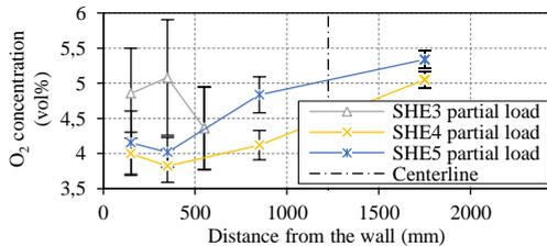
Fig. 7. O<sub>2</sub> concentration profile – air preheaters
