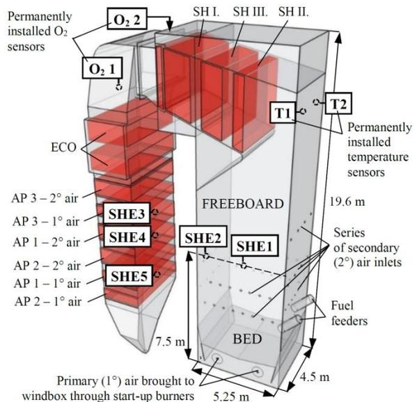
Fig. 1. Bubbling fluidized bed boiler 30.8 MW
