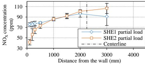
Fig. 5. NO<sub>x</sub> concentration profile – side walls of the furnace
