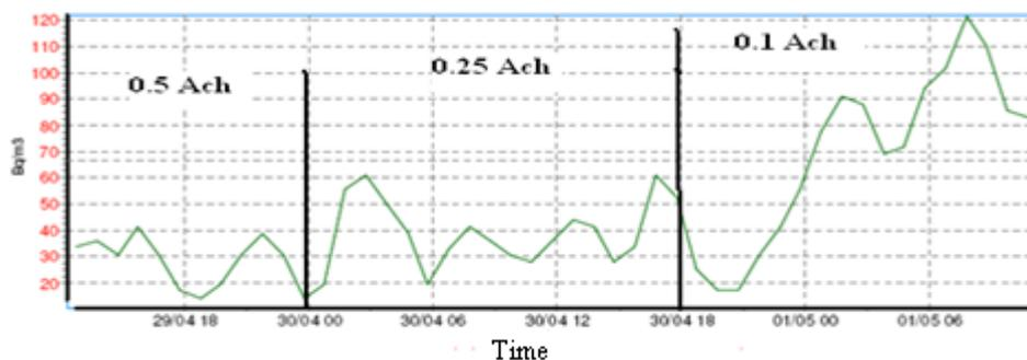
Fig.10. Measured radon level measurements versus ventilation rate
