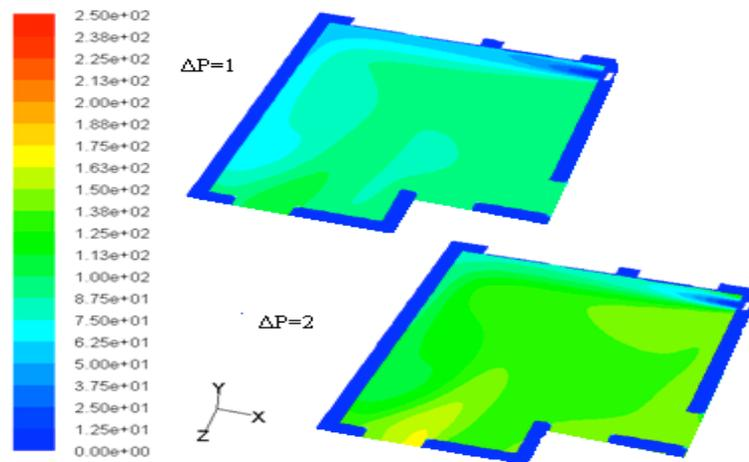
Figure 9. Contour of radon concentration for  $\Delta p=1Pa$  and  $2 Pa$
