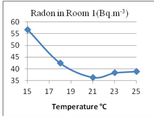
Fig.7. Radon concentrations in Room1 versus temperature
