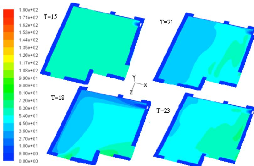
Figure 6. Contours of radon concentration in Room 1 at different temperatures
