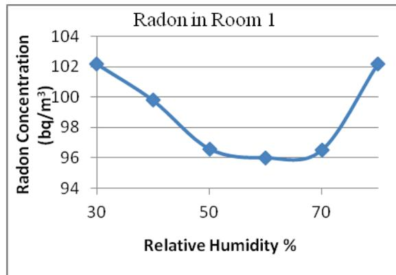
Fig. 8. Radon concentrations in Room1 versus relative humidity
