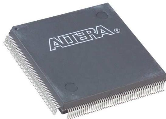
Is an integrated circuit containing identical logic cells (64 to 8'000 .000) which can be viewed as standard components. The logic cells are interconnected by a matrix of wires and programmable switches
