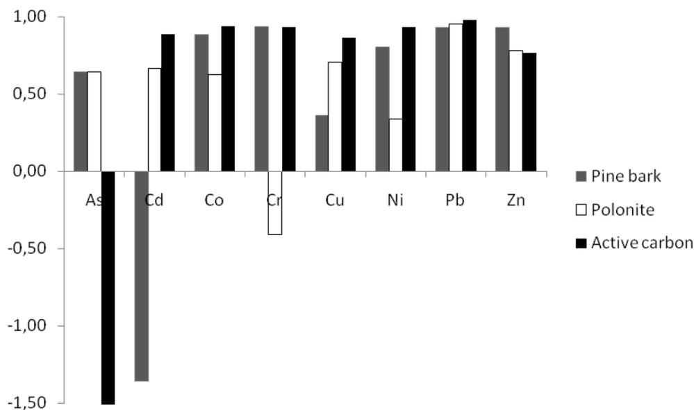
Figure 1 Relative treatment effect on the metal contaminated storm water of the three tested materials. Active carbon desorbed significant amounts of As, Polonite Cr and Pine bark Cd.
