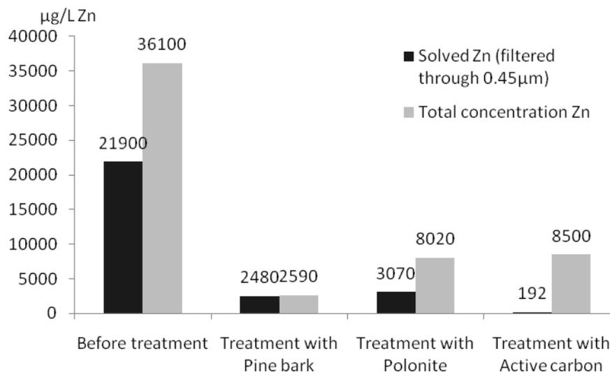
Figure 2 Concentrations of Zn in the untreated and treated storm water after filtration through pine bark, polonite and active carbon.
