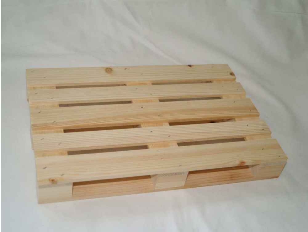
Figure 4. Wooden pallet (1:4 scale) used in the model scale tests.
