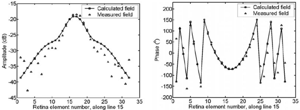
Figure 2 : Comparison between calculated and measured scattered field of a 35 mm PVC cylinder with a complex correction of the measured field.
