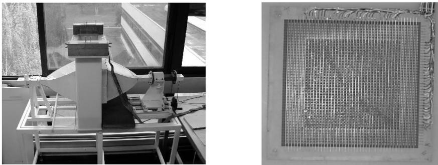
Figure 1: The 2.45 GHz microwave camera (left), the retina (right).
