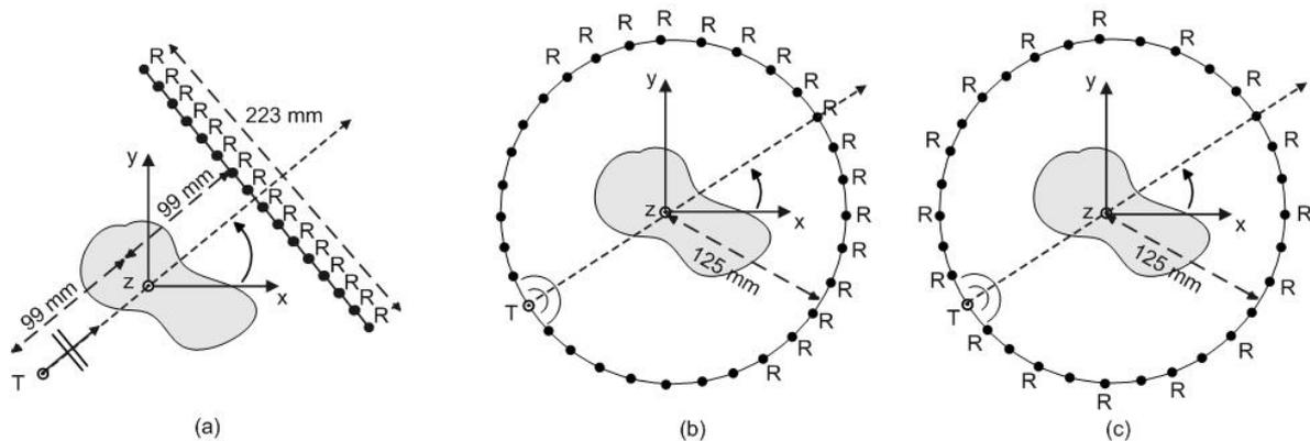
Figure 3 : The 3 different multi-view configurations. (a) Planar camera. (b) Barcelona camera. (c) Complete circular system
