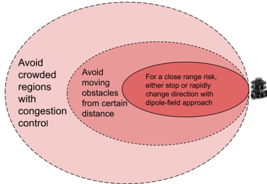
Figure 5.1: Multiple layers proposed to enhance path planning dependability.
