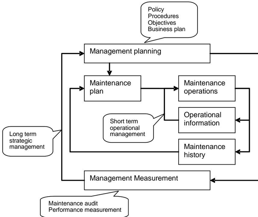
**Figure 8: The maintenance cycle (Coetzee, 1999).**
