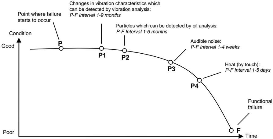
**Figure 6: The potential failure to failure curve of a ball bearing (Moubray, 1997).**
