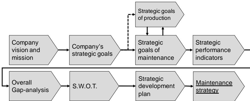
**Figure 13: A schematic view of the maintenance strategy formulation work-process (Appended Paper IV).**
