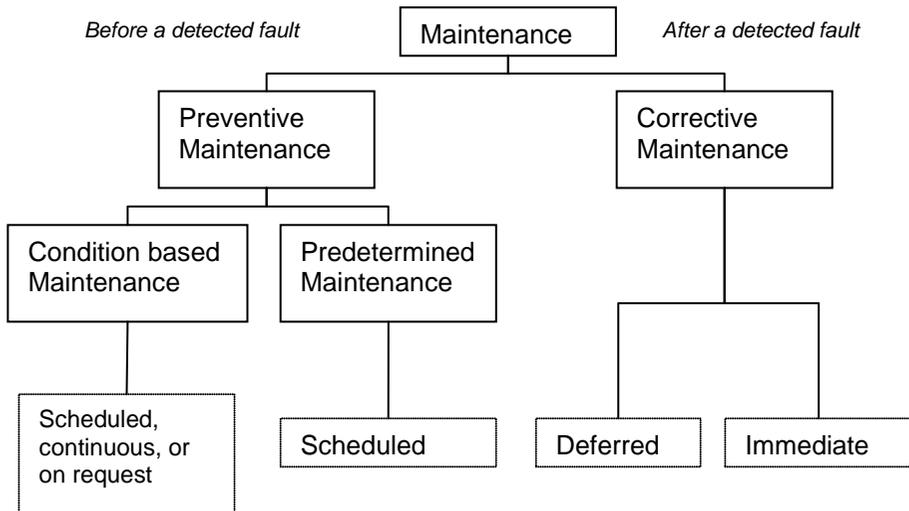
**Figure 5: Overview of different maintenance types (SS-EN 13306, 2001).**
