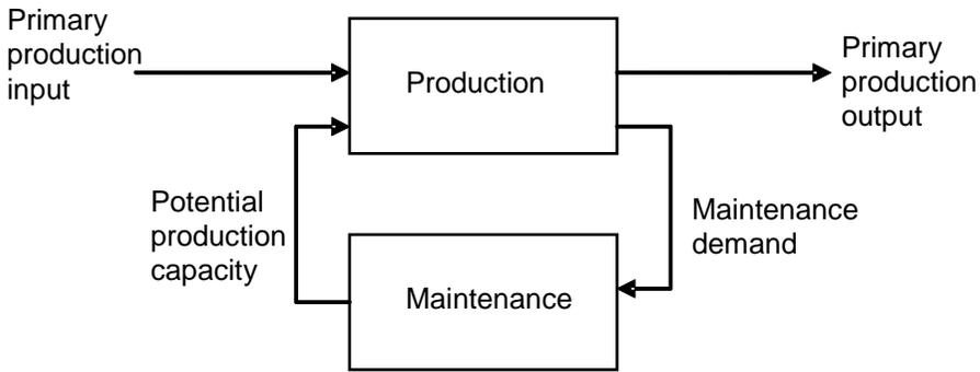
**Figure 4: The relation between Production and Maintenance (Gits, 1994). Maintenance demand is a secondary output from the production equipment, while maintenance results in potential production capacity as a secondary input to the equipment.**
