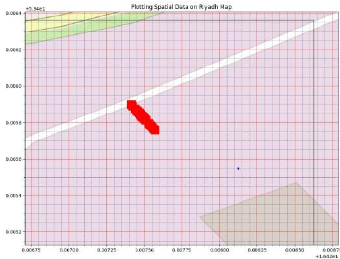
Figure 8: Gridmap where blue square is the UAV and the red squares are the detected objects. Straight upward is the North, while left is west, right east and down south. The compass angle from the UAV will be used to referee where the object are referring to the UAV. This is being static in the gridmap code, appendix C
