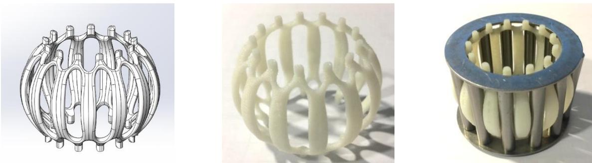
**Figure 28: Optimized holder. Shows CAD design, printed version, and printed version with all parts**
