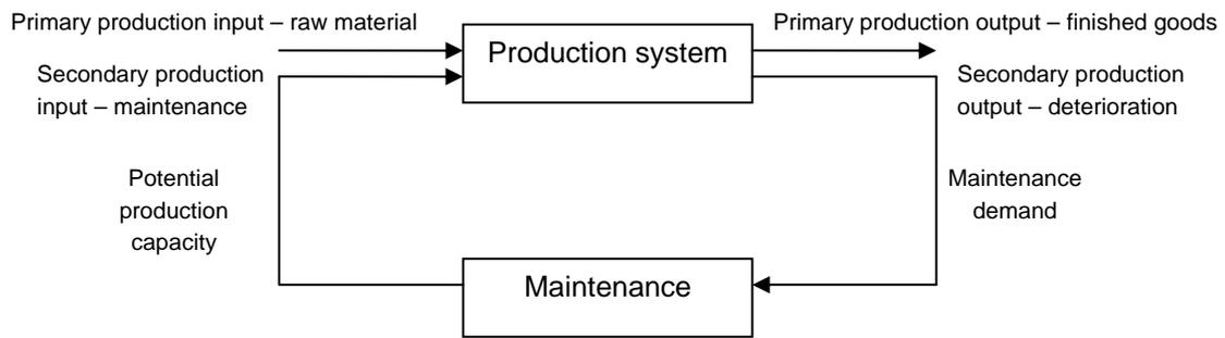
**Figure 6.** The need and affect of maintenance on a production system, adapted after Gits (1994). Obviously, additional support functions are necessary in order to run a production system. However, as the Figure visualizes, maintenance plays a vital role in upholding production capacity.
