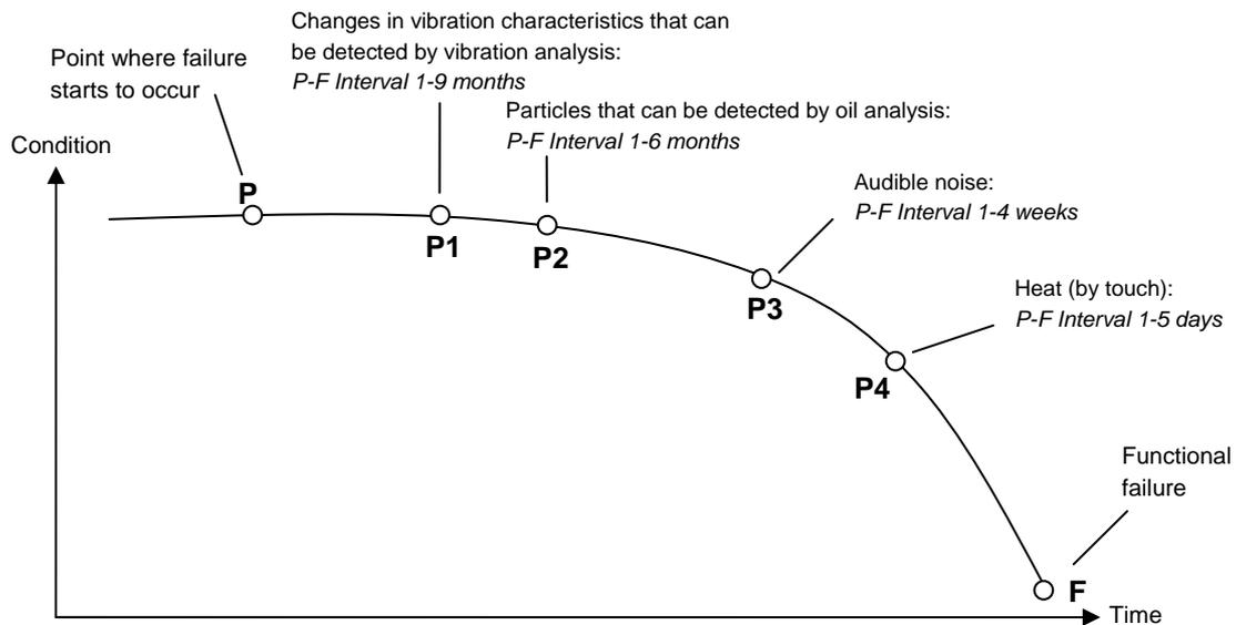
**Figure 4.** The potential failure to failure curve of a ball bearing (Moubray, 1997, p.144).
