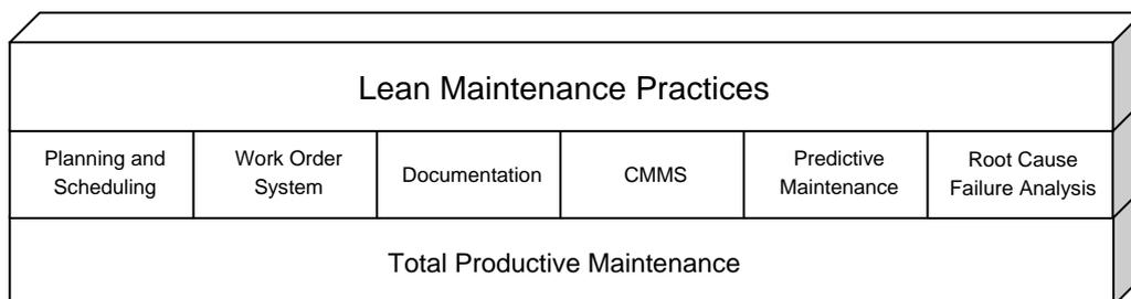
**Figure 9.** Lean maintenance practices, as visualized by Smith and Hawkins (2004, p.14). Total productive maintenance is the foundation, and six “bricks” achieve lean maintenance. CMMS is an abbreviation for computerized maintenance management.
