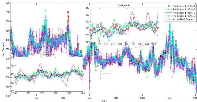
Fig. 1. Dynamic heat demand, predicted and measured results (in MWh)
