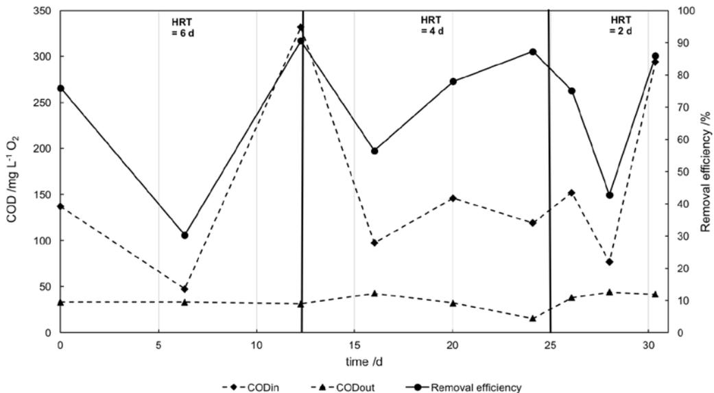
**Figure 3** Development of the chemical oxygen demand (COD) in the influent (COD<sub>in</sub>) and effluent (COD<sub>out</sub>) and COD removal efficiency at 6, 4 and 2 days hydraulic retention time during continuous operation of the microalgae-based activated sludge pilot plant.
