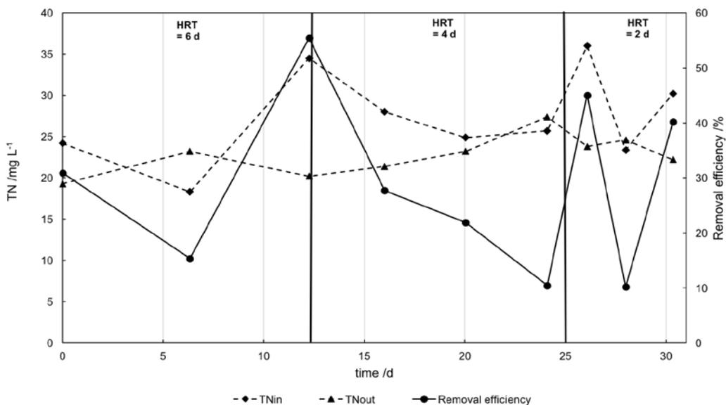
**Figure 4** Development of the total nitrogen (TN) in the influent (TN<sub>in</sub>) and effluent (TN<sub>out</sub>) and TN removal efficiency at 6, 4 and 2 days hydraulic retention time during continuous operation of the microalgae-based activated sludge pilot plant.
