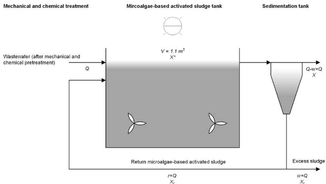
**Figure 1** Schematic setup of the microalgae-based activated sludge (MAAS) pilot plant.  $Q$ =discharge rate,  $w$ =ratio of excess sludge to discharge rate,  $r$ =ratio of return sludge to discharge rate,  $X^*$ =total suspended solids in MAAS tank,  $X$ =total suspended solids in effluent,  $X_r$ =total suspended solids in return sludge.
