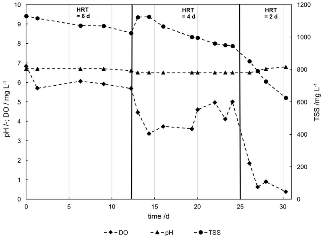
**Figure 2** Development of the pH-value, dissolved oxygen (DO) and total suspended solids (TSS) concentration at 6, 4 and 2 days hydraulic retention time during continuous operation of the microalgae-based activated sludge pilot plant.
