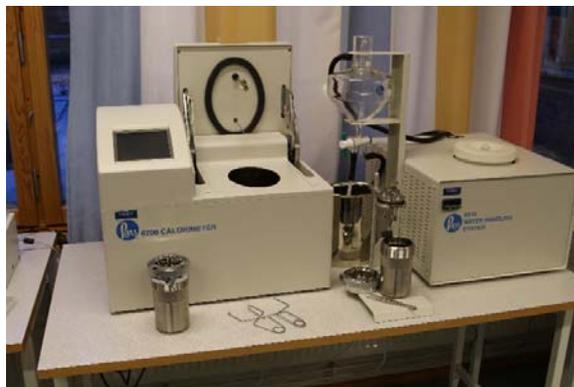
*Figure 7 Bomb Calorimeter*
